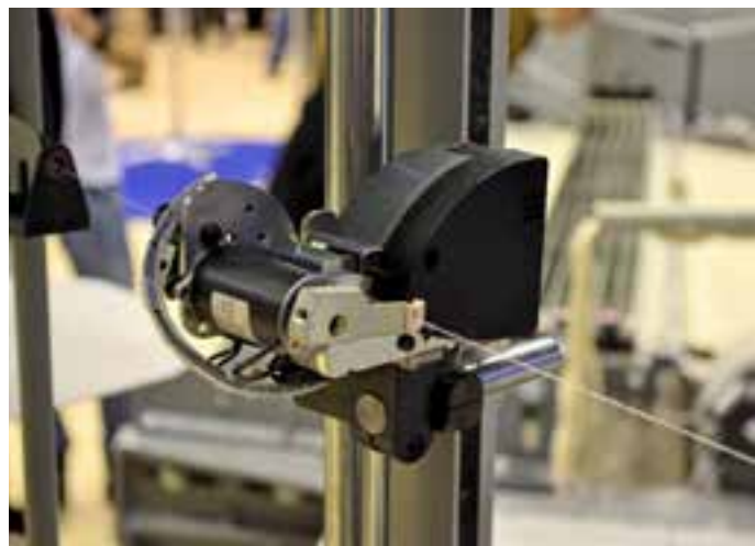
Sensor for fine-tuning air jets – a development by Toyota and Uster
