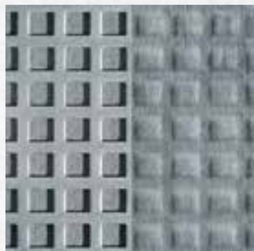
Detailed view of the structuring shell and the resulting thermobonded nonwoven
